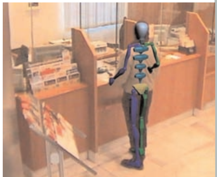
Scanned data superimposed with photo taken by observation camera - virtual people positioned in point cloud
